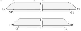
Put a slight curve front-to-back (camber) in all 4 wings.
